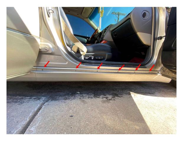
5. Drill out pre marked divets in the front and rear of the new kbd side skirts, install the hex head fasteners to the attachment points in the front wheel well and rear wheel well.
