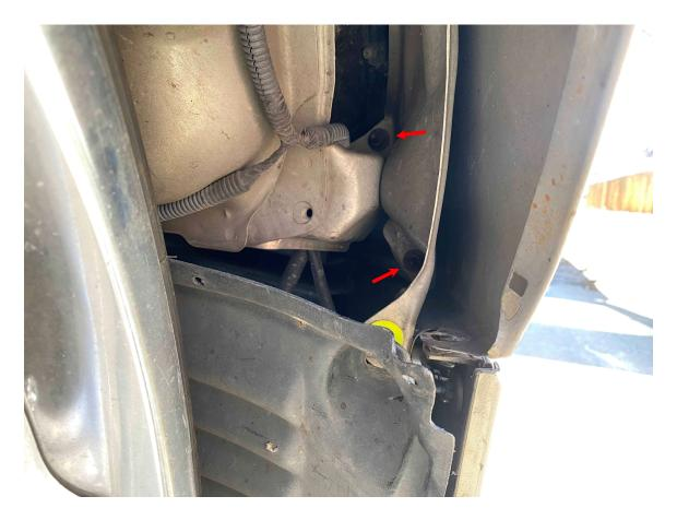
5. Remove the 8 fasteners underneath the front bumper that hold the bumper to the splash shield. (10mm)
