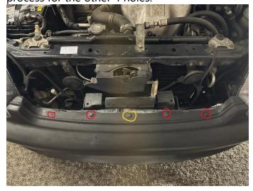
Final step is mounting the grill, place the grill onto the bumper and insert the 3 push pins that do not require drilling. Two on the core support and one on the bumper support. Now that the grill is secured, drill a pilot hole with the 11/64 bit for the mounting points on the top of the bumper following with the 3/8 bit. Now secure the grill with the final 2 push pins.
