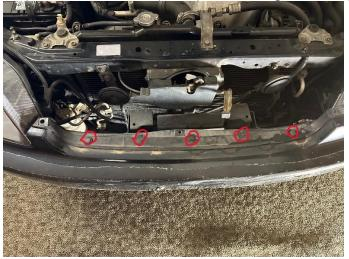
Step 5: Now you can remove the bumper and disconnect the side marker (will not be reused, use appropriate method to seal connecter from water), turn signal and fog light (if equipped).
