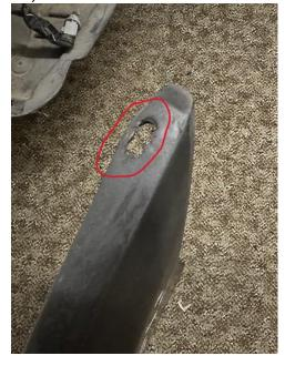
Step 3: Once the openings are cut reconnect the turn signal and fog light wires and slide the bumper onto the vehicle. Tap the bumper sides clipping the bumper to the fenders and install the screw leading to the fender.
