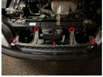
Step 4: Remove the 5 push pins holding the bumper to the bumper support bar.
