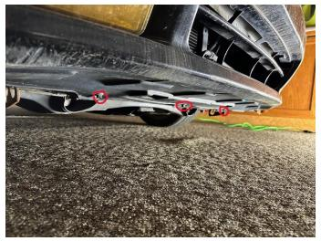
Step 3: Remove the 5 push pins from the grill then place it to the side.
