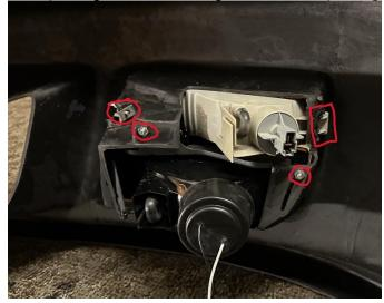
Step 2: The bumper has 3 indented locations on each side of the bumper where you must drill into the edges of each indent and cut the center out with a cutting tool to obtain best results. These 3 locations are identical to the openings on your factory bumper. 1 is for the screw holding the bumper to the fender (3/8 drill bit) and 2 openings are for the clips holding the bumper to the body (1/4 drill bit).
