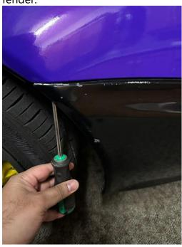
Step 2: Remove 5 10mm bolts connecting the bumper to the chassis (3) and fender liner (2).
